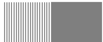
Figure 1: Image used to determine the angular resolution of the human eye
